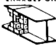
TNT PLACED ON ONE SIDE OF I BEAM
